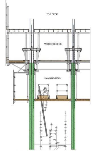
Picture 41: Typical scaffold stair tower access to slipform
