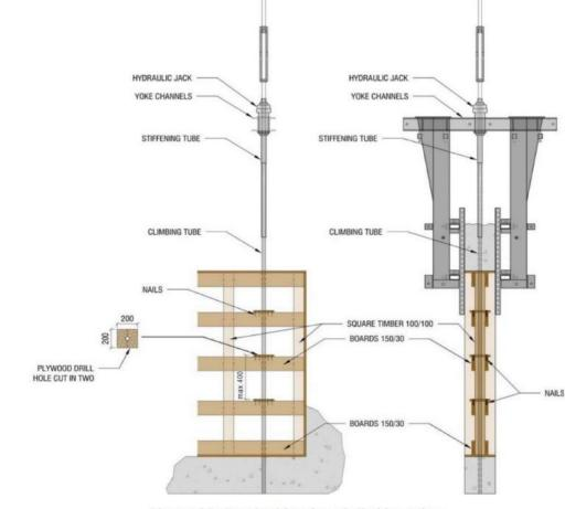
Picture 28: Standard bracing of climbing tubes
