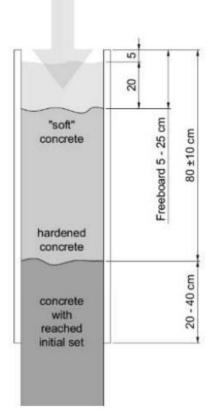
Picture 21: Setting of concrete in slipform
